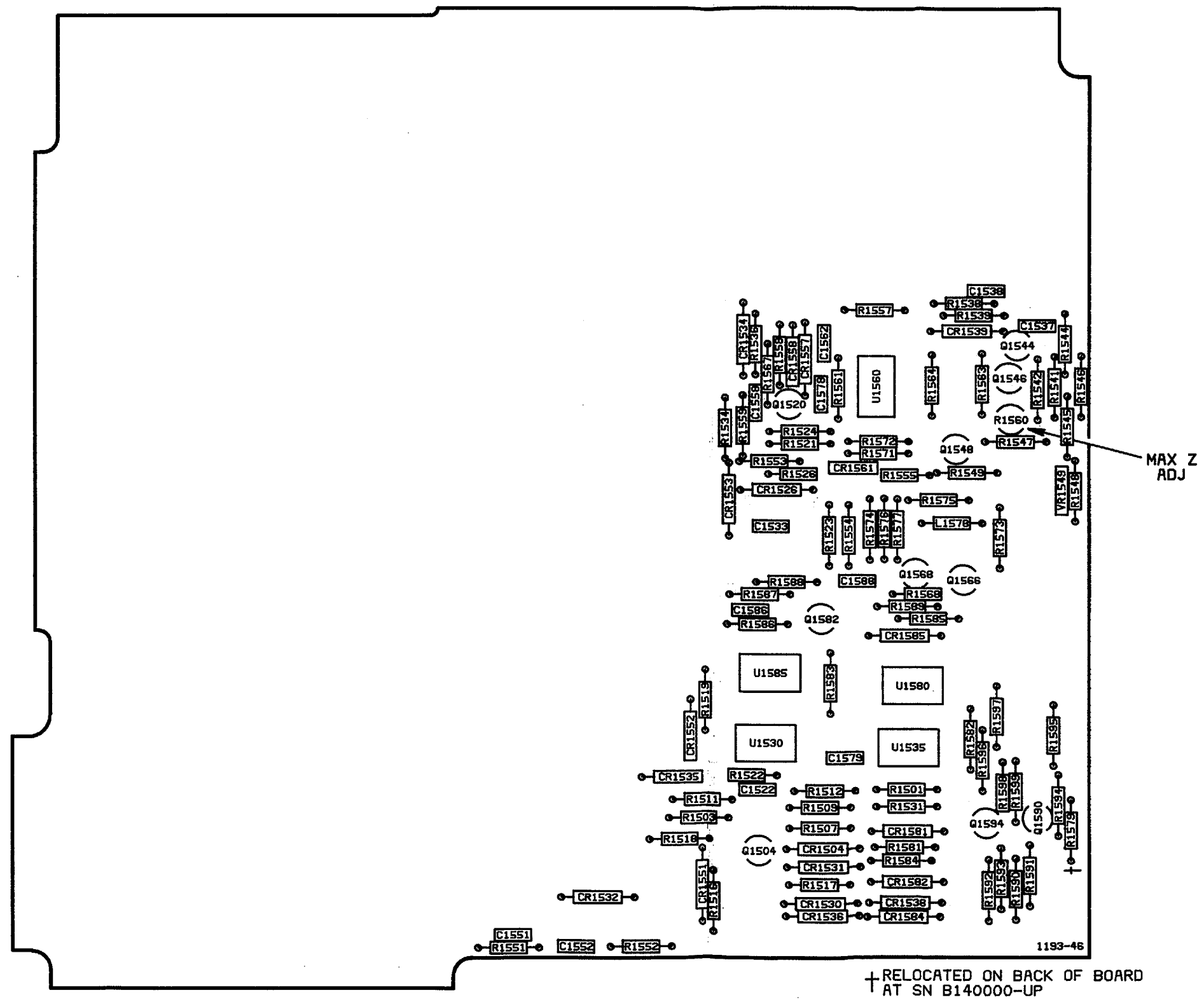
Fig. 8-14. A13 Partial Power supply board.
