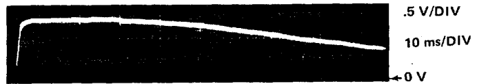
C.) At TP1951 Balance Node during sampling period then falling off due to short on -9 V supply.
